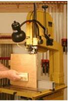
With the addition of our riser block kit, the PWBS-14 resaw capacity increases to 12" from the upper guide to the table surface!
